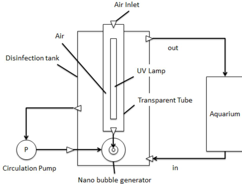
Schematic diagram of a Nano-bubble system
