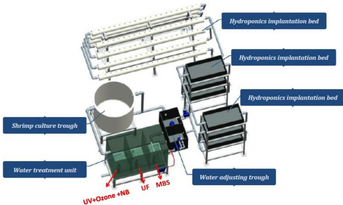
After the treatment in the system, ammonia concentration in the water could be reduced less than 0.5 ppm by MBS, moreover, greater than 90% of the common bacteria; around 99.9% of E.coli and Virus will be exterminated by UV+Ozone, and the Nano-bubbles will supply high oxygen content water for shrimps; meanwhile, debris in the water could be more easy to remove.
